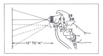
To obtain enough atomizing air, the available line pressure should be in the range of 60-90 psig. Use a 25-ft., 5/16"-minimum-diameter hose to avoid pressure drops in the line. The air compressor should be large enough to provide the volume and pressure required for all guns. It's important to control water and oil in the atomizing air since this will spot the paint and cause non-uniform distribution. Water and oil traps in the line will alleviate the problem.
